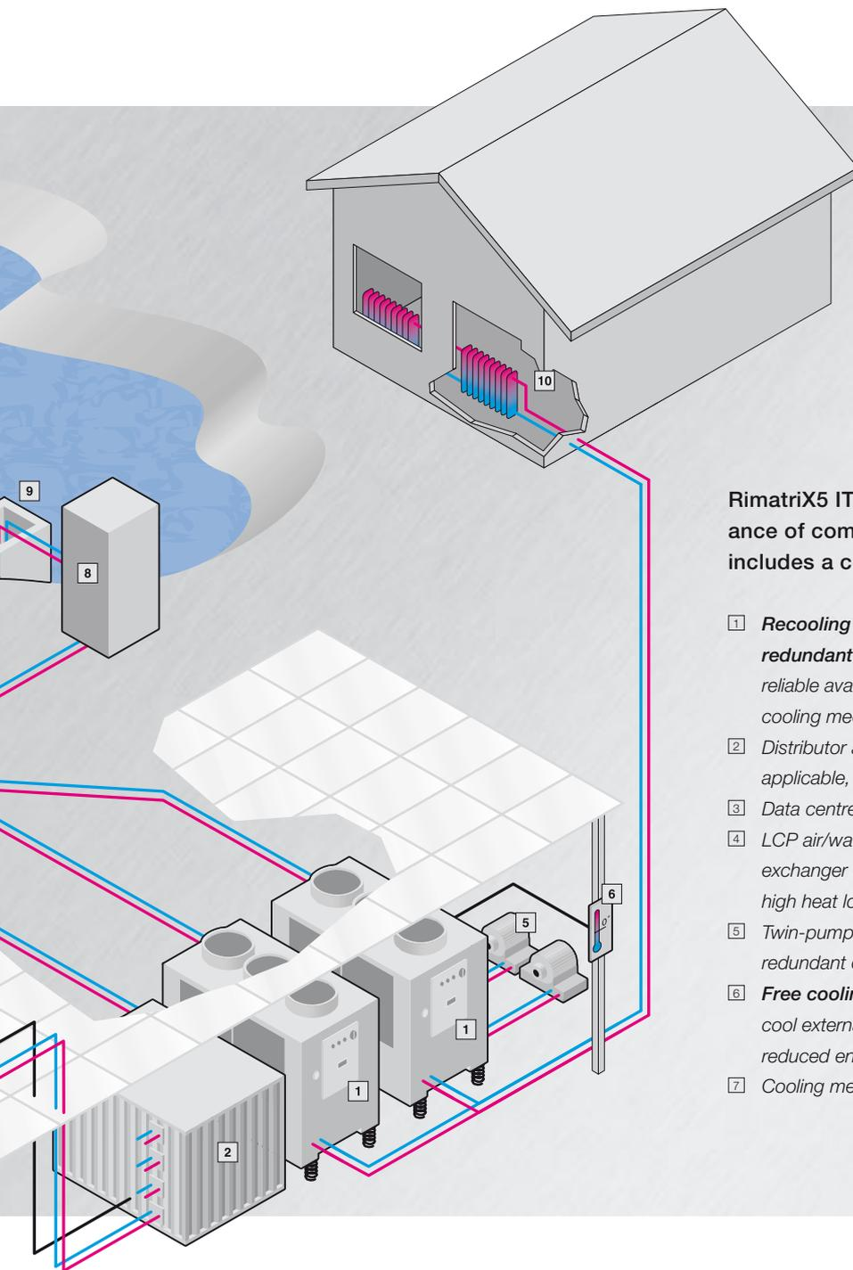
Rimatrix5 IT cooling systems offer the high performance of comprehensive system integration. This includes a complete pipeline network.
