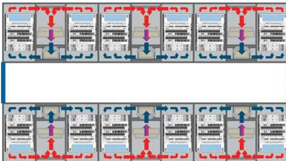
Direct rack cooling using Visiointec HDRCA series cooling units
